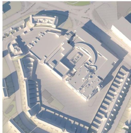
Shadows Cast at 4pm (UTC+0) on the 21 st March - Before Development Scenario
