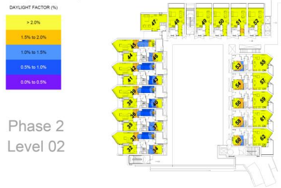
Figure 9 Daylight factor distribution diagram for rooms assessed at Level 02 in Phase 2 Development.
